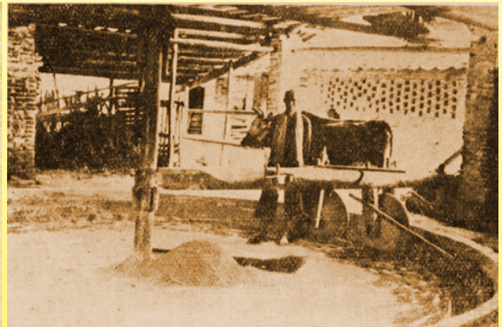
Grinding of kaolin by grinders powered by an ox (1939, Vietnam, Economic Bulletin of Indo-China)
